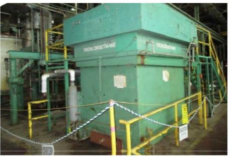
The vapor degreaser used trichloroethylene and later trichloroethane to remove oil and grease from equipment.
