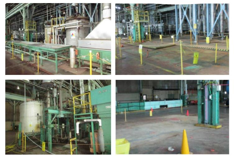
The alumina dissolver (above) was used to remove radioactive contaminants from activated alumina.
